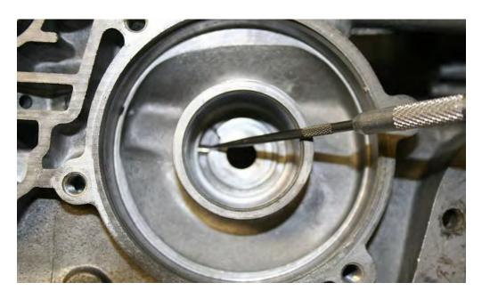
11. Flat file or wet stone entire channel passage area of case - absolutely no high spots or burrs allowed especially at area shown below.
