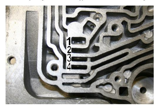
Brake On: Lands 3 & 4 are connected. Brake Off: Lands 2 & 3 are connected. Ensure solenoid plunger bottoms on solenoid back when stroked. Shims on bracket bolt may be needed when there is a shim on the solenoid.
