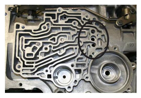
15. Reinstall low/reverse servo with new seal and steel gasket; *air check to ensure proper apply*.16. Modify stock modulator valve into brake valve as shown below.
