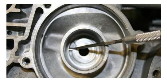
14. Flat file or wet stone entire channel passage area of case - absolutely no high spots or burrs allowed especially at center support case area shown below.
