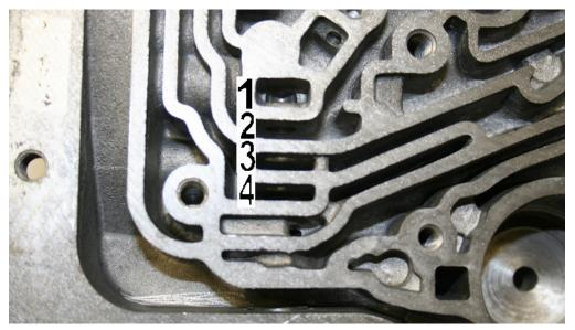
Brake On: Lands 3 & 4 are connected. Brake Off: Lands 2 & 3 are connected.
