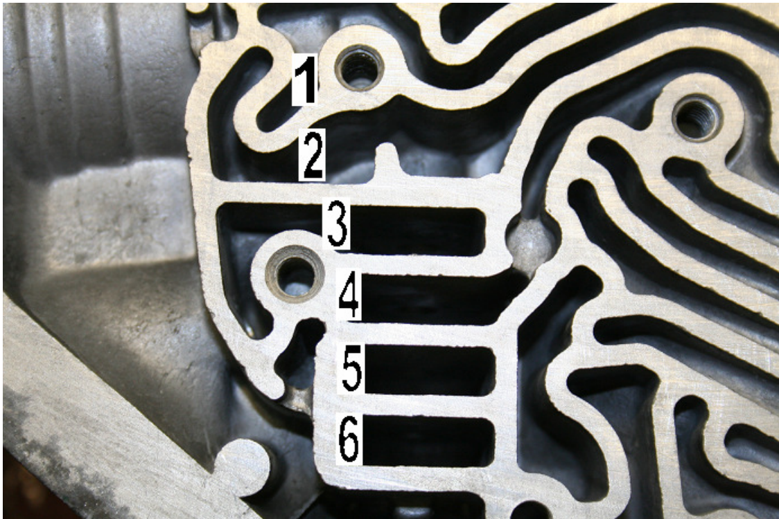
Figure 4 VALVE PHASE LOCATIONS BRAKE ON = 3 & 4 CONNECTED BRAKE OFF = 4 & 5 CONNECTED WITH SPOOL BORE OF MODULATOR VALVE
