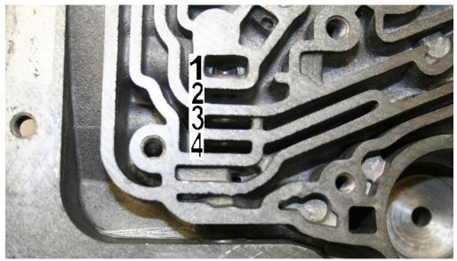
Brake On: Lands 3 & 4 are connected. Brake Off: Lands 2 & 3 are connected. Ensure solenoid plunger completely bottoms on solenoid back when stroked. Shims on bracket bolt may be needed when there is a shim on the solenoid.
