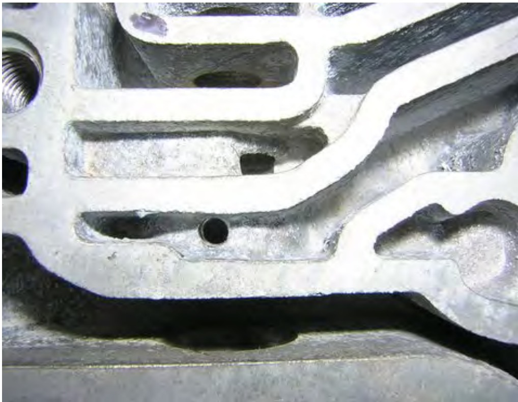
Figure 6 DRILLED HOLE THROUGH CASE & SLEEVE DO NOT DRILL THROUGH BOTH SIDES OF THE SLEEVE!
