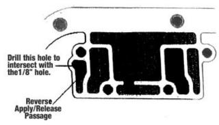
If you have an early model case (rear pump style) with the hole at the top of the piston area, follow these case modification details. Refer to the figure below. If the hole at the top of the case is drilled through the case, tap the hole 5/16-18 and install set screw below flush. Refer to the bottom of the figure below. Drill the additional lower hole all the way through using a 1/8" drill bit to create a pilot hole. Tap and plug hole with 5/16-18 set screw below flush.
